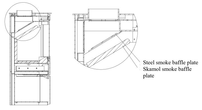
baffle plate is to be removed separately. Both smoke baffle plates are removed by lifting up at one side after which they may come clear at the other side and be taken down into the combustion chamber and out of the door. Similarly, they are put in place by leading them up slanting-wise at one side, and then at the other side, and they are then put into place in the middle.
