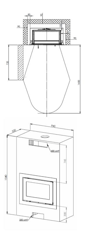
**Insulating material:** Useable are all AGI Q 132 registered insulating material. All measurements are intended as minimum distances.
