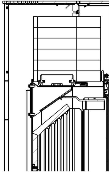
Each smoke baffle plate is to be removed separately. Both smoke baffle plates are removed by lifting up at one side after which they may come clear at the other side and be taken down into the combustion chamber and out of the door. Similarly, they are put in place by leading them up slanting-wise at one side, and then at the other side, and they are then put into place in the middle.
